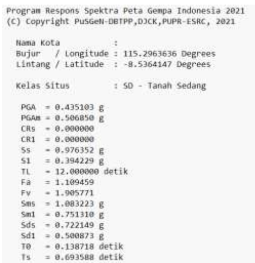
Figure 3. Output program response spectrum
