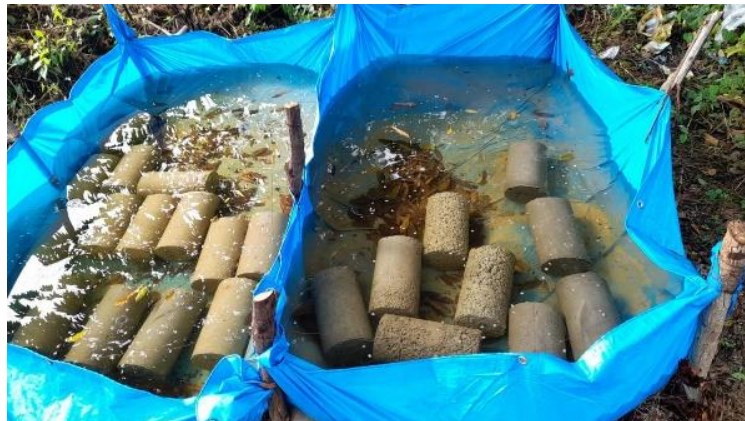
Gambar 5. Proses Curing Beton
