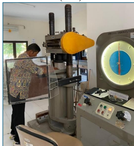
Figure 6. Compression Test Machine (CTM) testing
